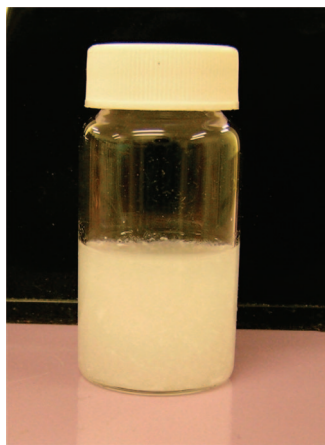
Figure 1. Photograph of 50/50 PVPh/PCL- b -P2VP complex formed in 1% (w/v) tetrahydrofuran (THF) solution.
